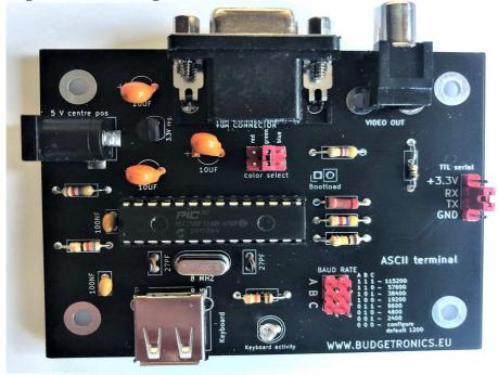
The baudrate jumpers are not really needed because you can also set the baudrate in the software, later more about this. On the PCB you can see how to set the baudrate with the jumpers. A number 1 is a jumper placed and a 0 is no jumper placed.
