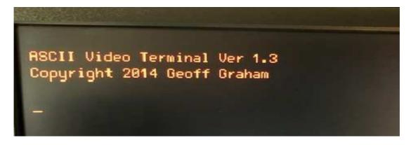
Gongratulations you suceeded building the kit successfully. If you place a jumper on the RX and TX header you can see the output of the keyboard if you press a key. This is just the echo and only used for testing because normally you will have an external data source.
